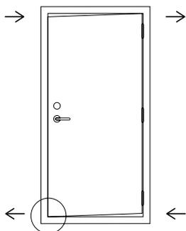
**The front part of the door leaf is rubbing at the bottom of the frame.**
