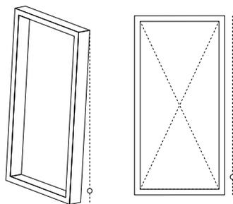
Check that the frame does not lean outwards or inwards, cross-measure carefully.
